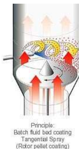
Fig 6: Tangential spray fluid bed coating
