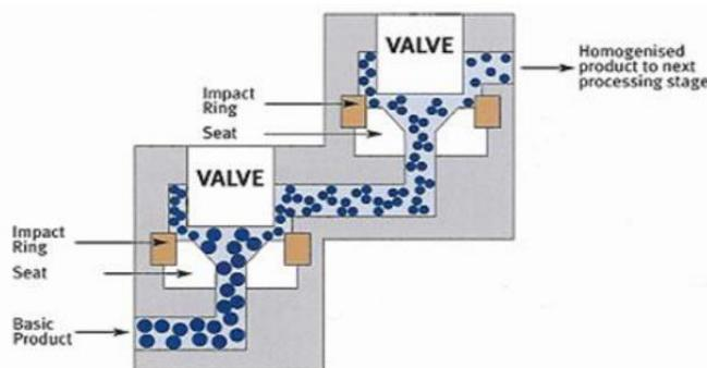
Figure no 2: High pressure homogenization
